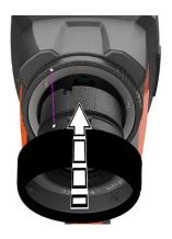
2 Align the markings on the lens and handle.
